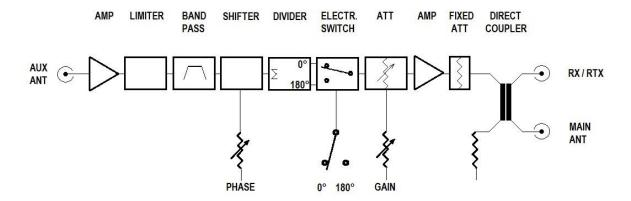
What this circuit reveals and amplifies, as in all "noise killers", is injected into the receive chain. It is therefore very important to not introduce any distortion or internally generated intermodulation products because they would inevitably be sent to the receiver.
